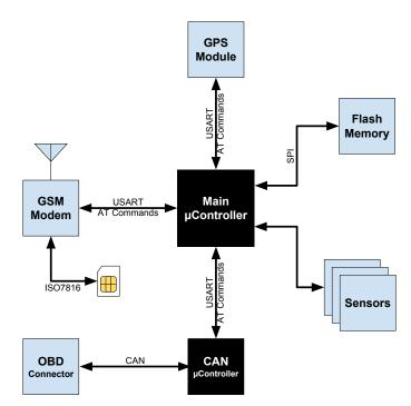
Figure 1. Example block diagram of dongle hardware
