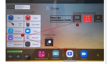
• If a participant in the room wants to connect wirelessly to the Cynap-Pro, the PIN can be displayed again on the (main) projector using the "Show mirroring info" icon.
